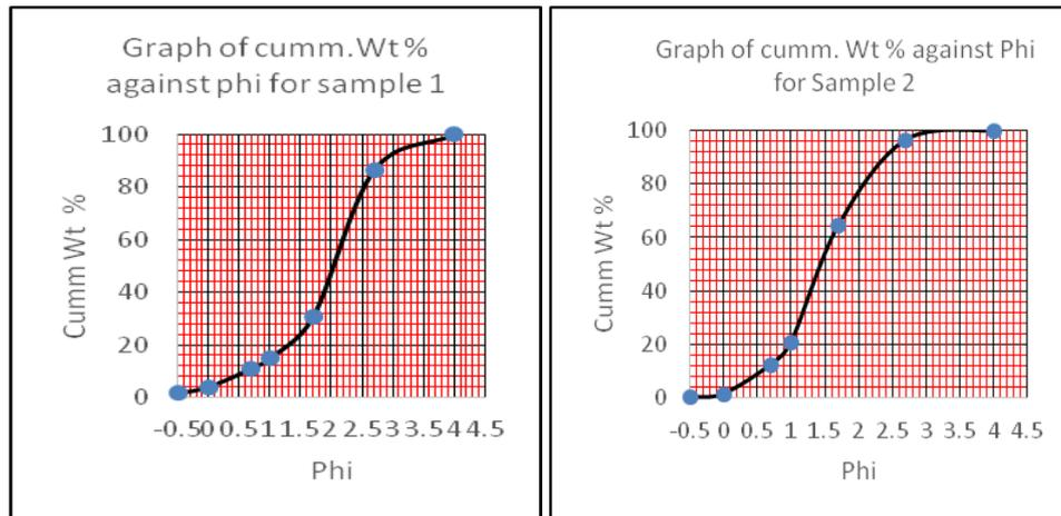
Fig : Cumulative frequency plot of Particle size distribution for samples 1 and 2
