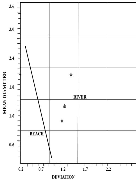
Fig. 4.6 Plot of mean size against standard deviation for sand-size particles of the study area (After Moiola and Weiser, 1968)
