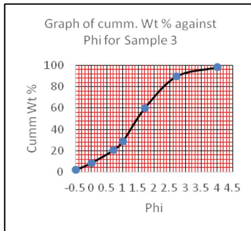
Fig : Cumulative frequency plot of Particle size distribution for sample 3
